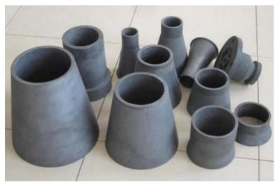
Reaction-bonded silicon carbide wear-resisting barrels are used for cyclone wear-resistant liner, instead of imported products, it has high strength, high wear resistance, good heat conduction performance.
